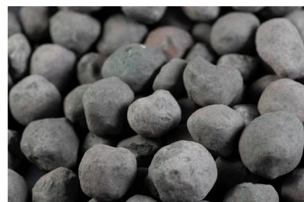
Abb. 121.3 Sinterpellets
